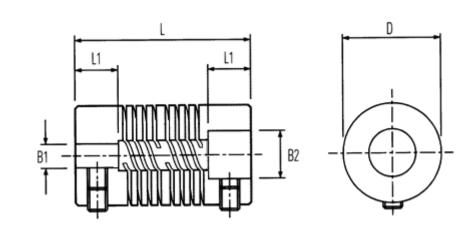
B1: Pre-drilled= 5.0B2: Pre-drilled= 8.00D= 25.4L= 38.1L1= 11.0Max angular displacement= 0.38Max B1 & B2= 12.00Max parallel displacement= 7
